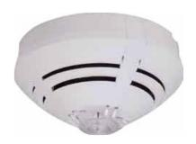
Multisensor detector with integrated optical detector and heat detector, with timecontrolled signal analysis and weighted data combination of both detector functions for detecting smouldering fires and fires with extreme heat generation. Intelligent detector with decentralised intelligence, self function test, CPU redundancy mode, automatic adaptation to the environments, alarm and operating data storage, alarm indication and soft addressing.
